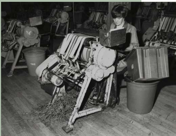
Worker at WD & HO Wills de-stemming leaf tobacco during cigar production, 1990. SC2535521. | Credit: © RCAHMS.
